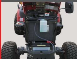
An extremely wide-opening hood provides good serviceability to the engine, air filter, and electrical components.
