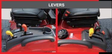
Various levers (HST Hi-Lo range shift, PTO select/clutch, etc.) are arranged either side of the operator seat in an optimal layout to ensure comfortable operation.
