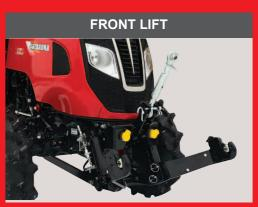
Front lift cat. 1 with a lifting capacity of 1000 kg.
