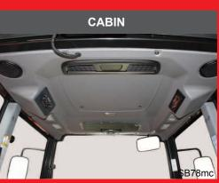
Nicely finished, low-noise factory cabin, standard with radio and air conditioning.
