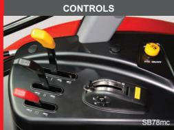
Electro-hydraulic controls are ergonomically designed for convenient operation.
