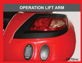
The 3-point lift arm control buttons are positioned on the rear fender under the rear light.
